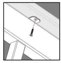
Install two (2) #10 x 3/4" Square Drive Flat Head screws in each plate through countersunk holes and into deck board. Continue this process until all deck board cap rails are installed.
