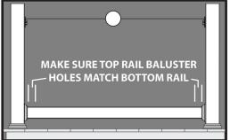
**TOP RAIL - Measure between black mounting** brackets. If post is plumb, top rail should be same length as bottom rail. Make sure distance from baluster pocket to post on each end is the same for both top and bottom rail.
