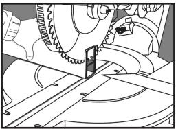
Cut top rail including aluminum insert to length to match bottom rail. Cut vinyl rail and aluminum reinforcement at the same time.
