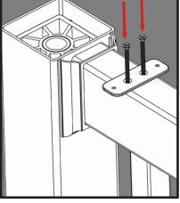
Install two (2) aluminum mounting plates on top of rail 2" from each post with two (2) #8 x 2-1/2" Install remaining two (2) aluminum mounting plates at quarter points on top rail. Deck board cap rail should be installed only after all of the 2" x 3-1/2" rail sections have been installed.
