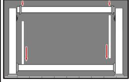
Slide pre-cut bracket trim ring on both ends of top rail. Insert end balusters into top rail and be sure rail slides down into black mounting brackets side guides.
