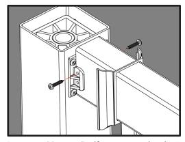
Insert one (1) #10 x 1" self-tapping pan head screw through black mounting bracket and into vinyl rail and aluminum insert.
