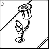
3. Strip the insulation back ½" from the 18-2 gauge wires and the LED Surface Mount Light LED feed wires. Using the supplied waterproof wire nuts connect the wires. Note: Polarity must be maintained. Always connect the same side of 18-2 gauge wire with the same polarity (i.e. positive) marked on the LED Surface Mount Light wires. LED Surface Mount Light feed wires are 60" long.
